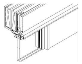
**Curtain Wall** is a high performance aluminum framed wall system typically containing both vision glass and opaque metal or glass spandrel panels. These systems are supported by brackets, attached to the floor slabs and typically run entirely outside the structure, past the slab edge.
