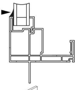
**Casement Window** is an operable window with a vertically hinged sash to open in, or more usually out.
