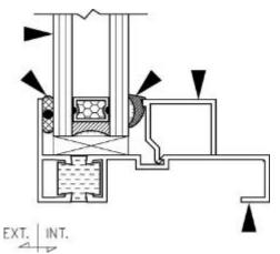
**Awning Window** is an operable window with a top mounted hinged sash that swings out at the bottom.
