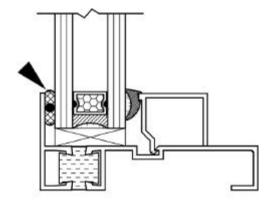
**Window-Wall** refers to the use of traditional residential windows adapted for floor to ceiling use. They are typically supported directly on the slab rather than outside the slab edge.
