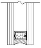
**Interface** refers to a location within the building envelope where two different components or assemblies meet. This could be two different wall assemblies or a wall and a window assembly.
