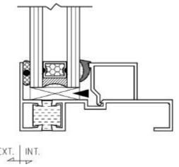
**Shear Block** is a type of joinery that uses an extruded or cold-formed shape (the shear block) that is attached to a vertical mullion to reinforce a corner of a sash or frame. The horizontal member fits over the shear block and is secured by screws driven into the shear block.
