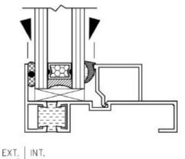
**Face Seal** refers to a strategy for rain penetration control that relies on the elimination of holes through the cladding or outer surface materials to limit water ingress.
