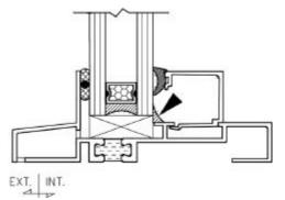
**Hopper Window** - is an operable window with a bottom mounted hinged sash that swings in or out at the top. (similar to an awning window, except hinged at bottom).
