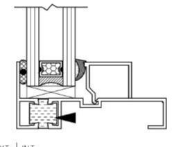
**Threshold** is the lower horizontal member of a doorframe extending from jamb to jamb that lies directly under a door and is set on the floor.
