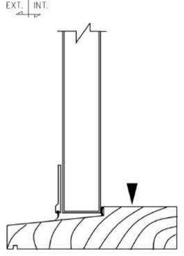
**Through-wall Flashing** refers to a waterproof membrane or metal flashing placed under segmented precast concrete, stone masonry or brick units known as copings that close the tops of masonry walls to prevent water from entering the wall at joints in the coping. Through wall flashing is also used to prevent capillary transfer of moisture through porous materials such as concrete or masonry if they extend from high moisture locations such as below grade.
