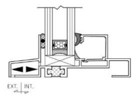
**Drip Flashing** directs water flowing down the face of vertical elements, such as walls or windows, away from the surface so that it does not continue run down the surface below the element.
