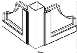
**Coupling Bars or Adapters** are a special extrusion, tube or specific shape to assemble two individual window frames together, either vertically or horizontally, creating a composite window.
