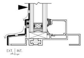
**Weatherstripping** refers to material around operable lites used to reduce air leakage or water penetration, or both.
