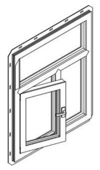
Glass Bite is the amount of overlap between the stops and the edge of the glass.
